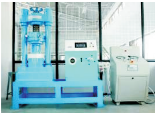
UKL Gasket Test Laboratory showing machines for testing compressibility, recovery and sealability.
