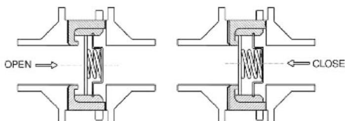
The Non-Slam Check Valves get opened by the pressure of the fluid and get closed by the Spring as soon as the flow ceases.
